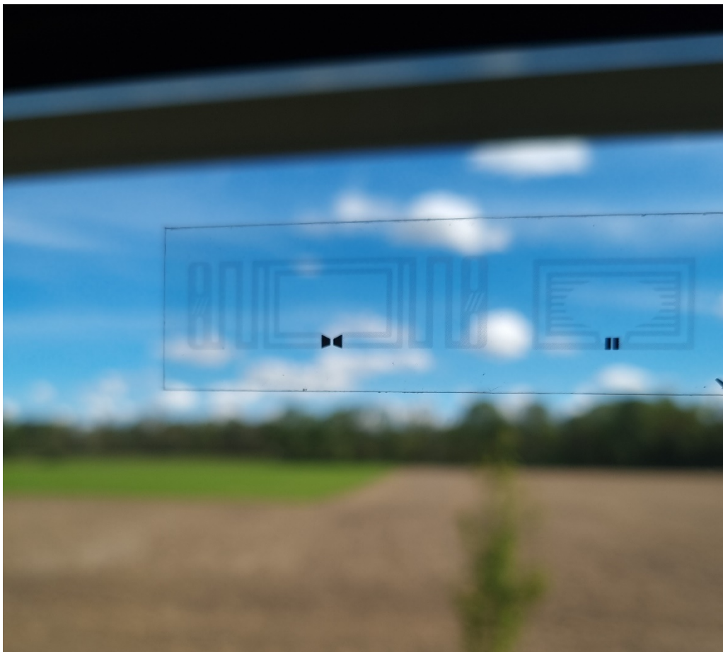
Fig. 4: View on (and through) transparent RFID antennas.
